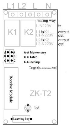
Assuming the transmitter is coded 2262 or 1527 chip encoder chip remote control.
