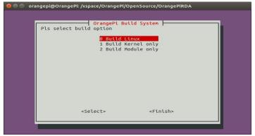
This version is only support the above three options. After selecting the corresponding option, the system would compile automatically.
