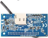
• Make sure the toggle switch is showing like the following, booting from SD card.
