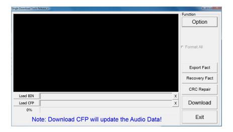
Click "load BIN" to import the image of NAND version into writing tool. After that, click Download button to download the image. Meanwhile, the tool is waiting for the download link of Orange Pi i96.
