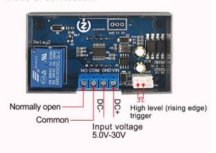
4.PNP sensor signal trigger—mode of connection:
