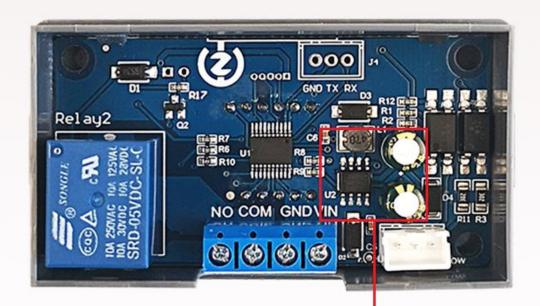
DCDC buck circuit supports 24 V No heating, No burning, Upgrade the old LDO circuit
