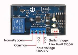
3. High level (rising edge) signal triggering — mode of connection:
