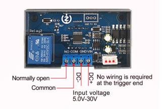
2.Passive switch signal trigger— mode of connection:
